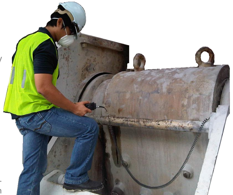
Acquiring vibration data from a jaw crusher using a data collector
